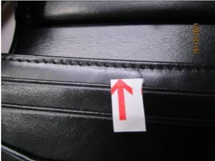
DEFECT 6: BULGING SURFACE
