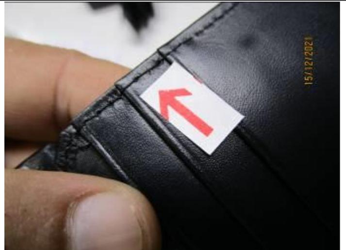
DEFECT 1: BROKEN SEAM
