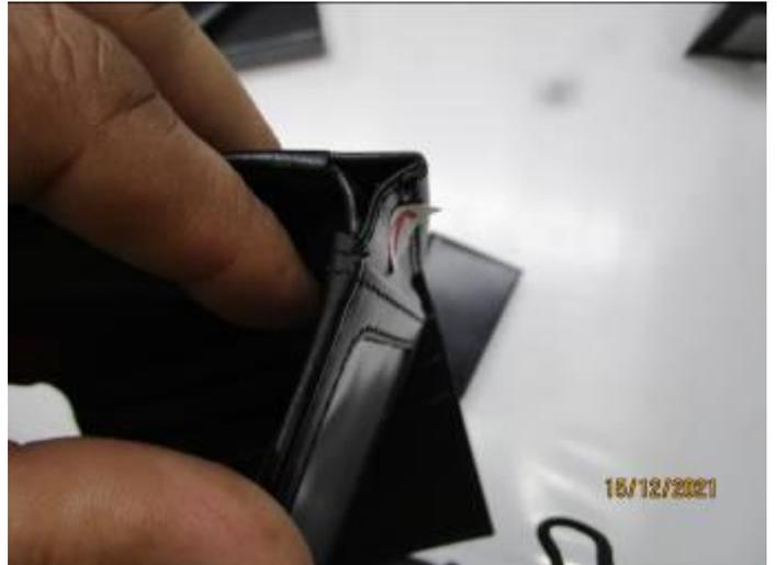
DEFECT 6: INSECURE EDGE JOINT
