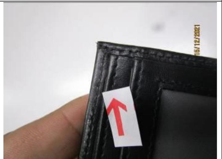
DEFECT 1: BROKEN SEAM
