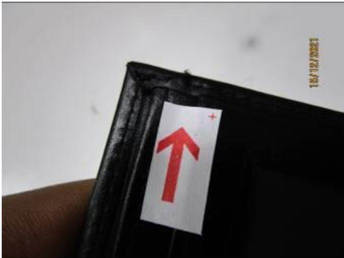
DEFECT 2: BROKEN SEAM
