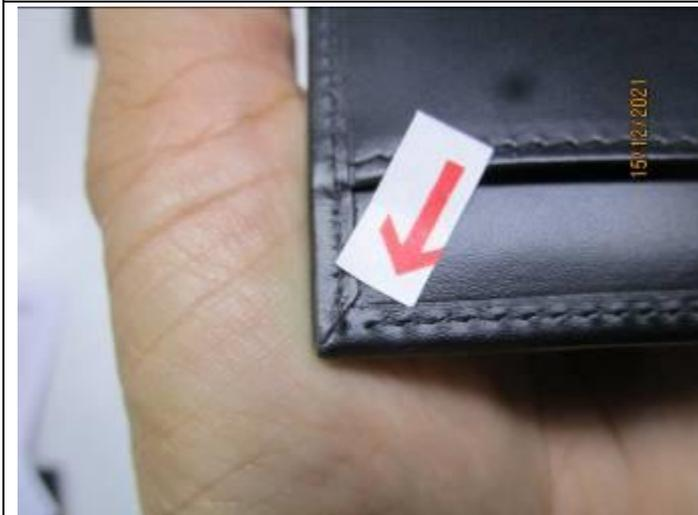
DEFECT 3: BROKEN SEAM
