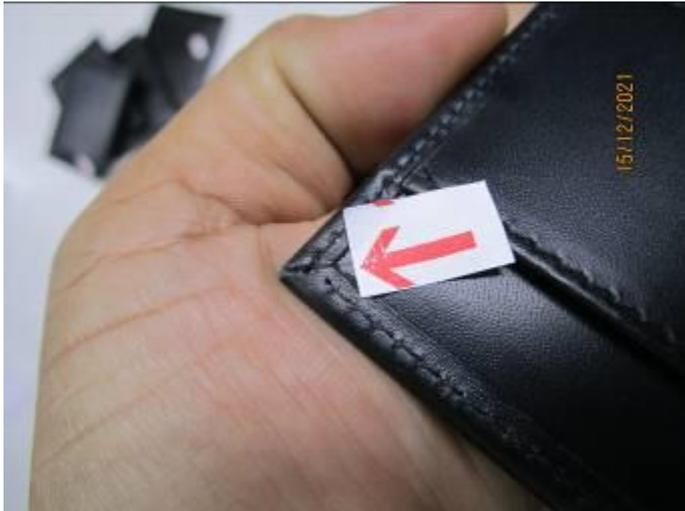
DEFECT 5: BROKEN SEAM
