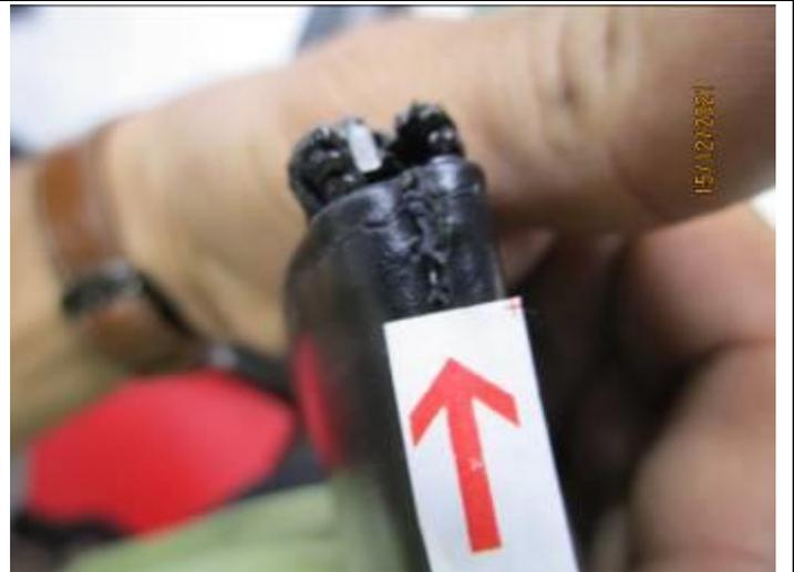
DEFECT 1: IMPROPER MANUFACTURING
