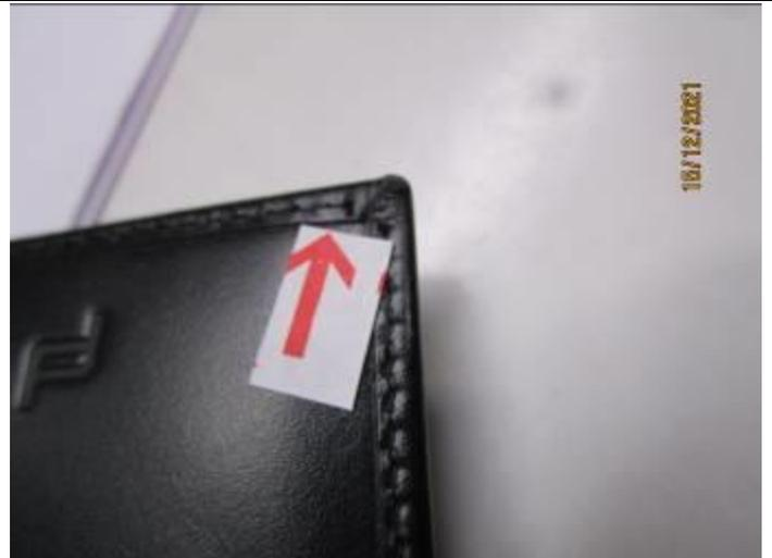
DEFECT 3: BROKEN SEAM
