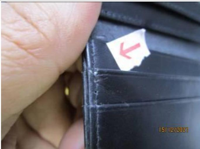
DEFECT 4: CUT LEATHER DUE TO NEEDLE HOLE
