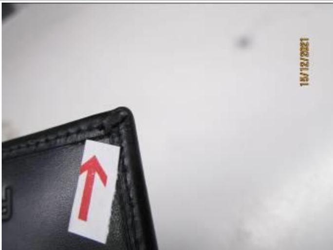
DEFECT 4: BROKEN SEAM
