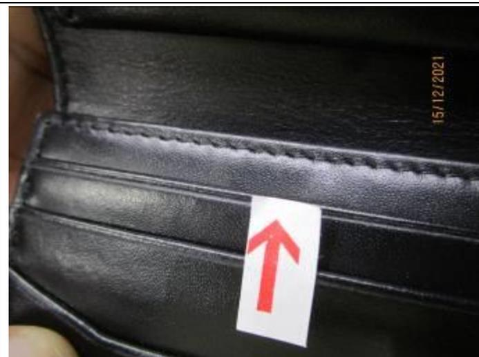
DEFECT 2: BULGING SURFACE
