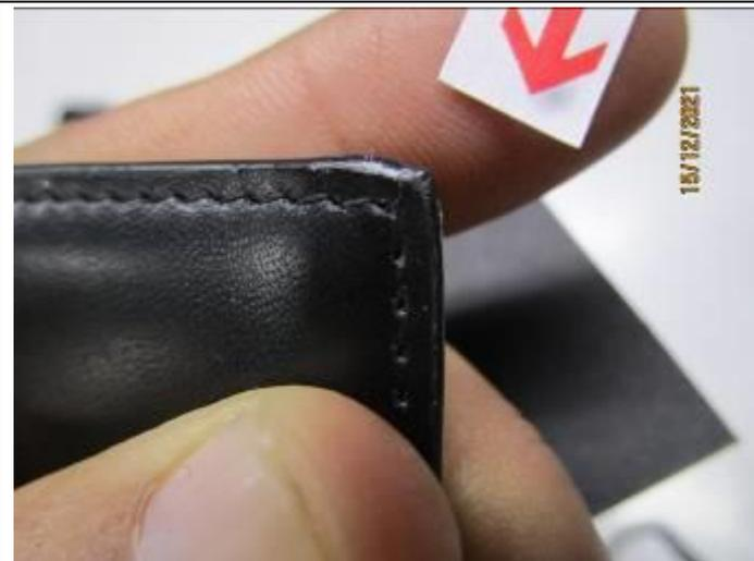
DEFECT 2: IMPROPER EDGING
