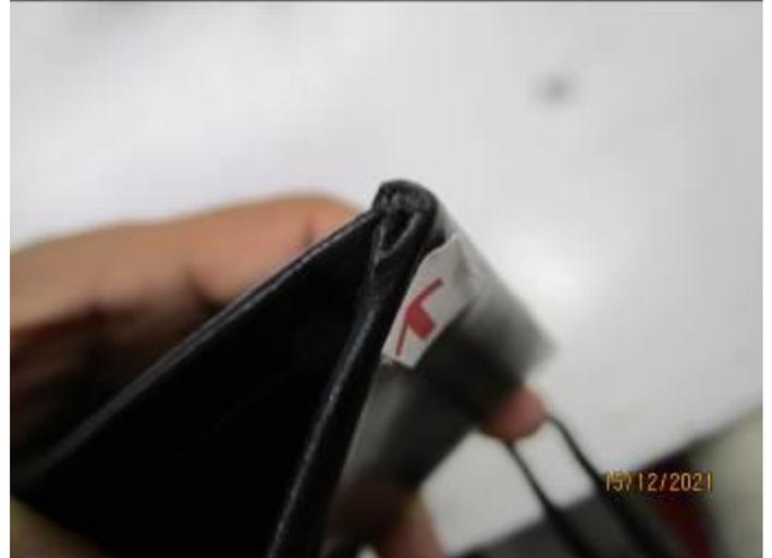
DEFECT 3: IMPROPER EDGE LOCKING
