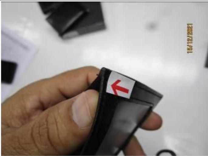
DEFECT 7: INSECURE EDGE JOINT
